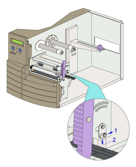
Figure 6-4, Print Head Balance Adjustment
